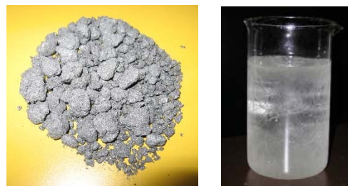
Figure 7 Sodium acetate with graphite (left) and paraffin RT27 (right)
